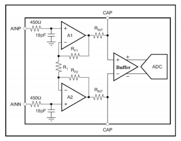
Figure 4: PGA structure diagram
