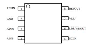
Figure 2: CS1237 Chip Pinout
