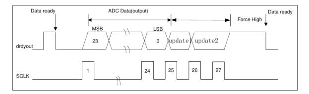
Figure 8: Read data timing diagram 2
