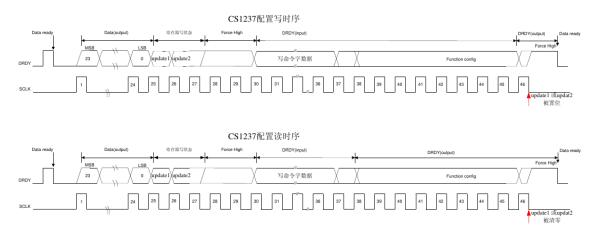
Figure 9: Function configuration timing diagram
