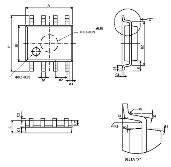
Figure 11: Chip SOP8 Package Size Information
