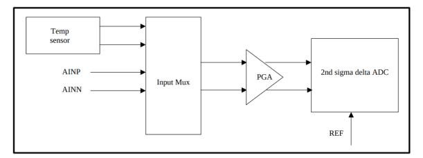
Figure 3: Analog input structure diagram
