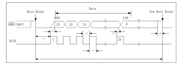
Figure 7: Read data timing diagram 1
